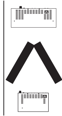
Fig. 1 Device may be mounted before or after A-coil in either horizontal or vertical air handling systems.
